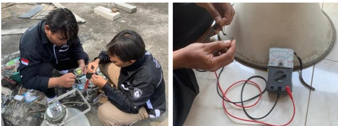
**Gambar 2.** Pengecekan Kondisi Spul Speaker TOA ZH-5025BM
